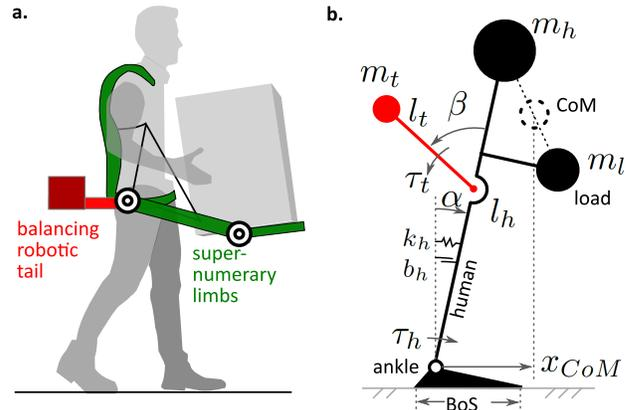
Fig. 1: **a:** a user carrying a load assisted by the supernumerary limbs and the balancing robotic tail. **b:** the mechanical model used for simulation.
