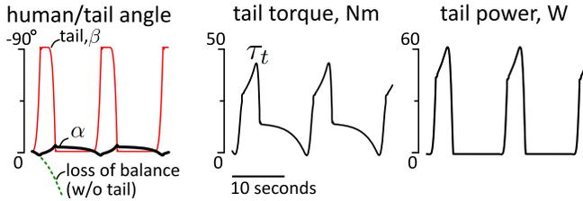
Fig. 2: Simulation results. Time histories of human's and robotic tail's angular orientation (left), torque produced by the tail's controller (middle), and power produced by the tail (right). The dashed green line on the left plot corresponds to the simulation test without the robotic tail (unstable case, rapid loss of balance is observed). All plots have the same time scale (total simulation time was 30 seconds).
